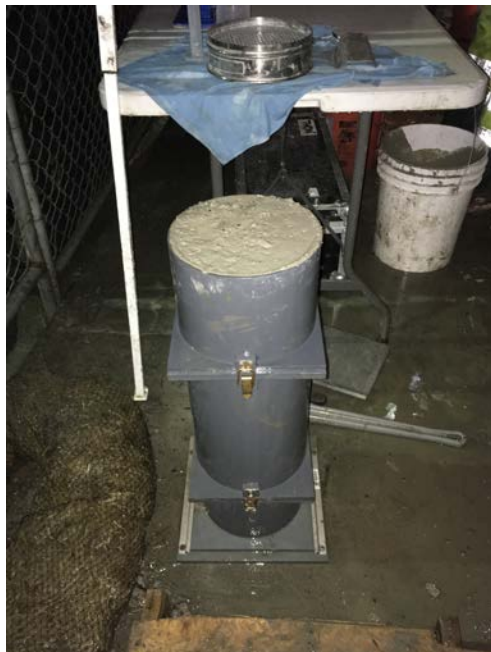
Figure A.5: Arrangement for static segregation test in accordance with ASTM C1610
