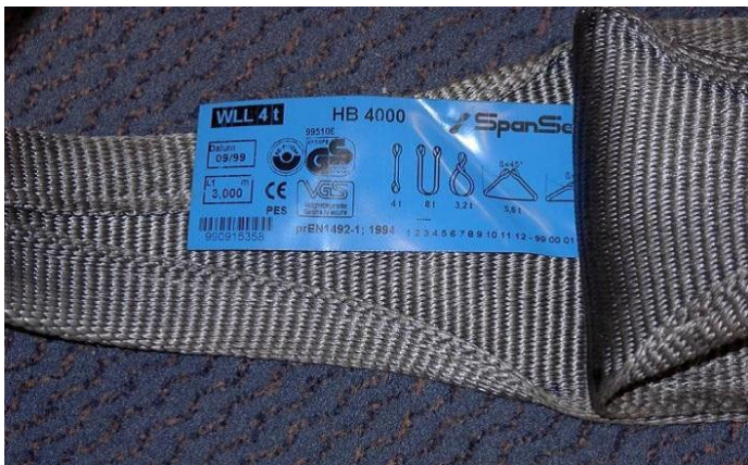
Picture 1: Multiple use polyester (PES) webbing sling according to DIN EN 1492-1 – blue label
