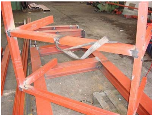
Picture 8: Single-use slings sharp edges
