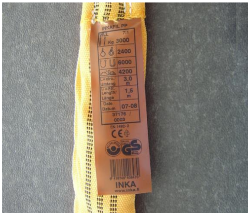
Picture 2: Multiple use polypropylene (PP) round sling according to DIN EN 1492-1 – brown label
