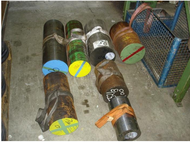
Picture 7: Single-use slings – use in production
